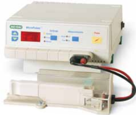
MicroPulser electroporator with cuvette chamber attached. Electroporator is shown connected to the assembly cuvette.
